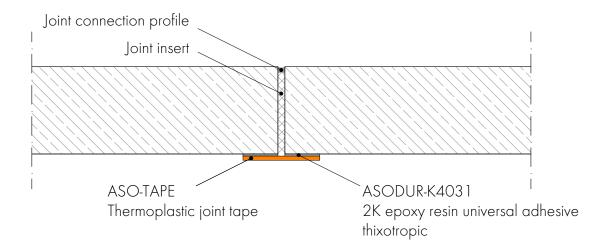
Overlap area ASO-TAPE / watertight concrete >5cm up to 2bar and >20cm with water pressure 2 to 5bar
