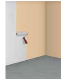
7 Application of the primer on the wall
